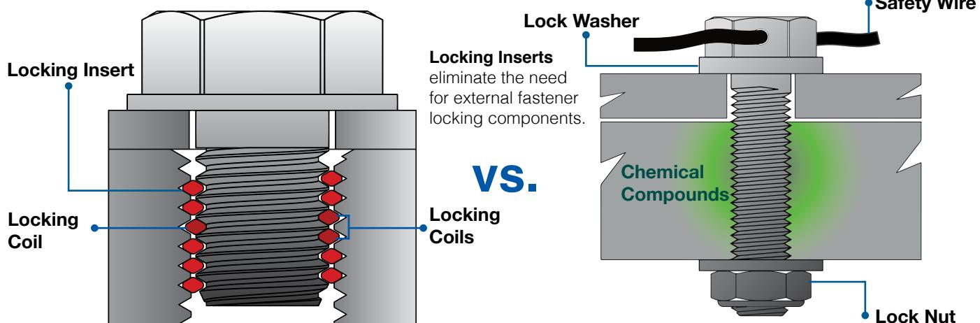
KATO screw locking inserts exert a prevailing torque on male threaded fasteners to prevent loosening due to vibration or impact. Locking inserts eliminate the need for costly and less desirable locking mechanisms. They are excellent in adjusting screw applications by preventing the male fastener from creeping.
