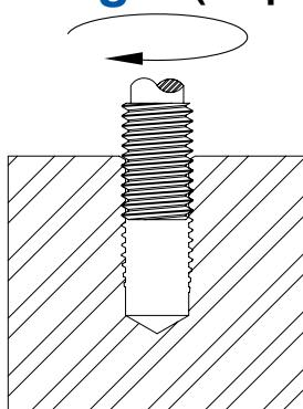
CoilThread® STI Plug Gauges (page 51) are used to check the major and pitch diameters of the STI tapped holes. Gaging the tapped hole prior to insert installation is critical to ensure the accuracy of the finished thread. If the tapped hole gauges correctly, the installed CoilThread® insert will be within the thread tolerance. No further gaging is necessary. If gaging is attempted after the
