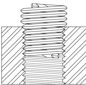
Follow the instructions accompanying the KATO installation tool for proper insert installation. Insert installation depth is dependent on the presence of a countersink (3/4 to 1-1/2 turns below the surface with a countersink and 1/4 to 1/2 turns below the surface without a countersink).
