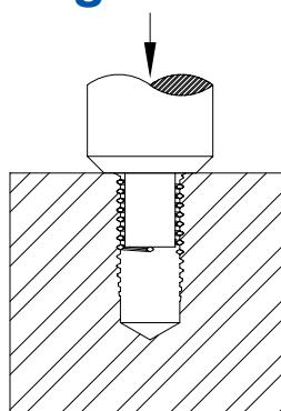
KATO recommends the tang always be removed to ensure that the full threads of the bolt fully engage the locking coils (when using locking inserts). To achieve maximum assembly strength the bolt must engage the entire insert length. Use the KATO Tang Break-off Tool (page 83) to ensure accurate and clean tang break off. In blind holes it may be necessary to remove the broken tang from the bottom of the hole (recommended).
