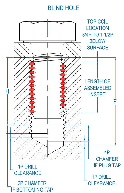
1. Standard size drills are suggested even though some sizes vary slightly from the minor diameter specifications in MA1567.
