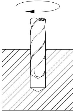
The drill sizes shown are recommendations only, based on expected material behavior for increased tap life in harder materials. Actual individual conditions may require varied drill sizes in order to produce the correct minor diameter after tapping. For example, compensation must be made in tolerances for plating.
