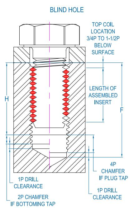
1. Standard size drills are suggested even though these sizes vary slightly from the minor diameter specifications in NASM33537.
