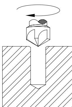
The "F" and "H" values (pages 14-17) are calculated with a countersink depth of 1/2 pitch.
