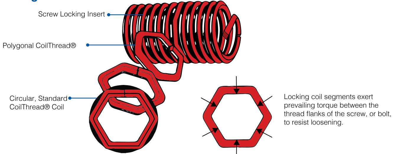
One, or more, of the coils in the insert have a series of straight segments. Upon entry of the bolt these straight segments are flexed outwardly, creating pressure on the bolt. This pressure is applied between the flanks of the bolt thread so that contact area is maximized and unit pressure is minimized. It is often possible to realize cycle life far in excess of specification requirements (15 cycles).
