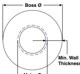
The recommended boss diameter is two times the STI tap major diameter max. For most materials, a minimum wall thickness equal to the nominal bolt diameter may be used when measured from the centerline of the hole (min boss diameter equals two times nominal thread size).
