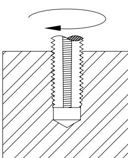
Tap using CoilThread® STI Thread cutting taps (page 41). The pitch diameter limits shown tabulated on pages 15 & 17 conform to NASM33537 and/or MA1567 respectively, and must be met in order to assure proper thread fit after installation of the CoilThread® insert.
